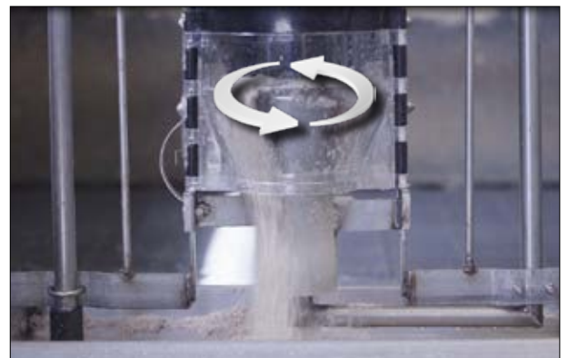
Feed automatically fills when sensor indicates the empty trough.
