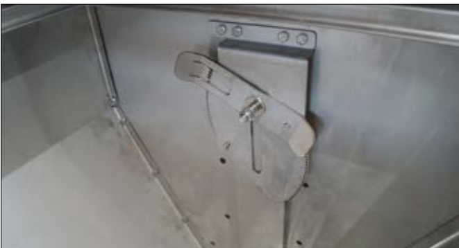
The adjustment system requires only two adjusters per feeder, providing quick, accurate and consistent control of feed gate settings.
